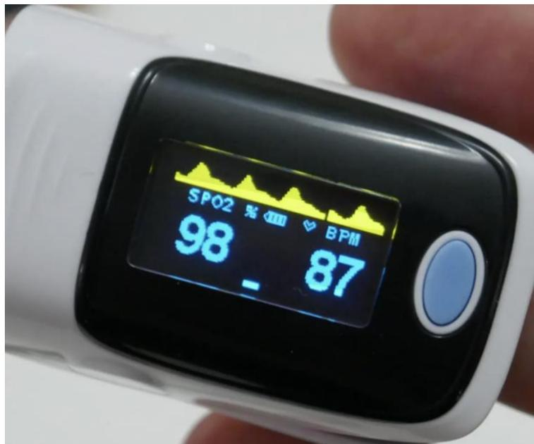
The number under BPM (“87”) is the heart rate. And if the waveform (yellow lines at the top) are consistently rising and falling with each beat, that is how you know the tool is working correctly.
